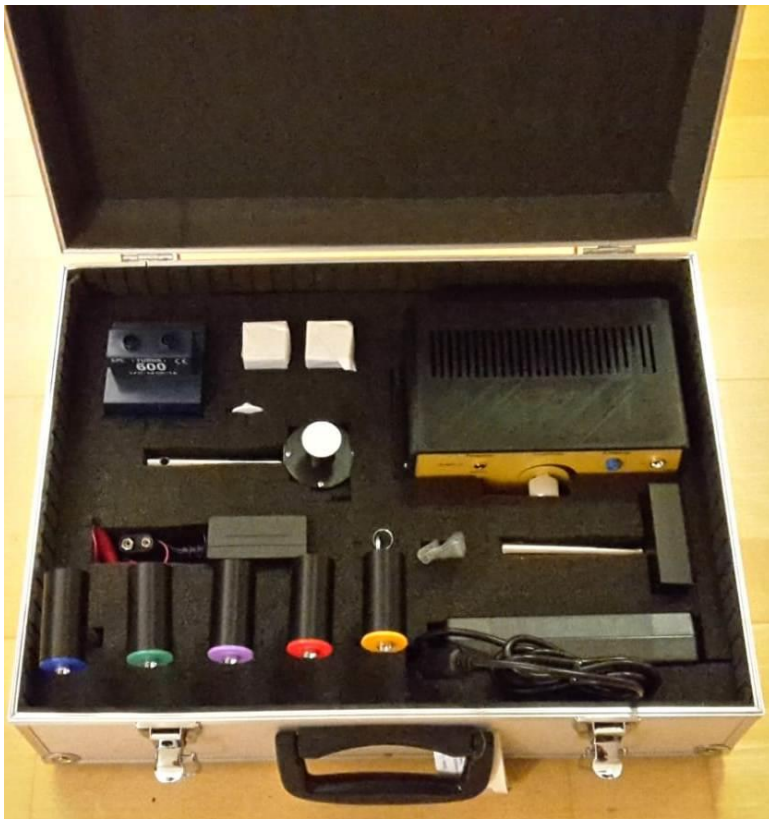
Faraday Rotation Kit – Basic (laboratory experiment)
