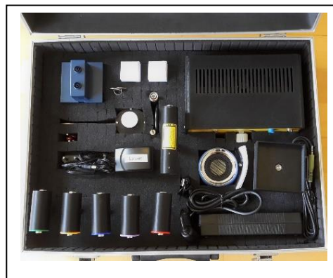
Extended Kit “Faraday Rotation including additional lecture hall demo: Free Space Information Transfer“
